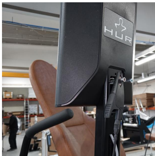
Figure 3, One of the display's fixing screws is used as one measurement point.
