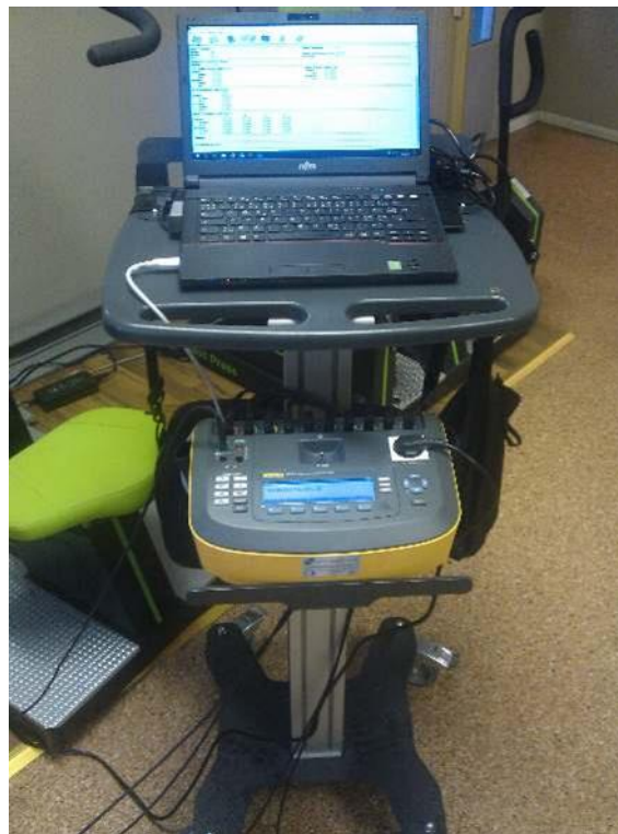
Figure 1, At the factory the machines are tested using a Fluke ESA620 controlled by the Biomedical Test View software.
