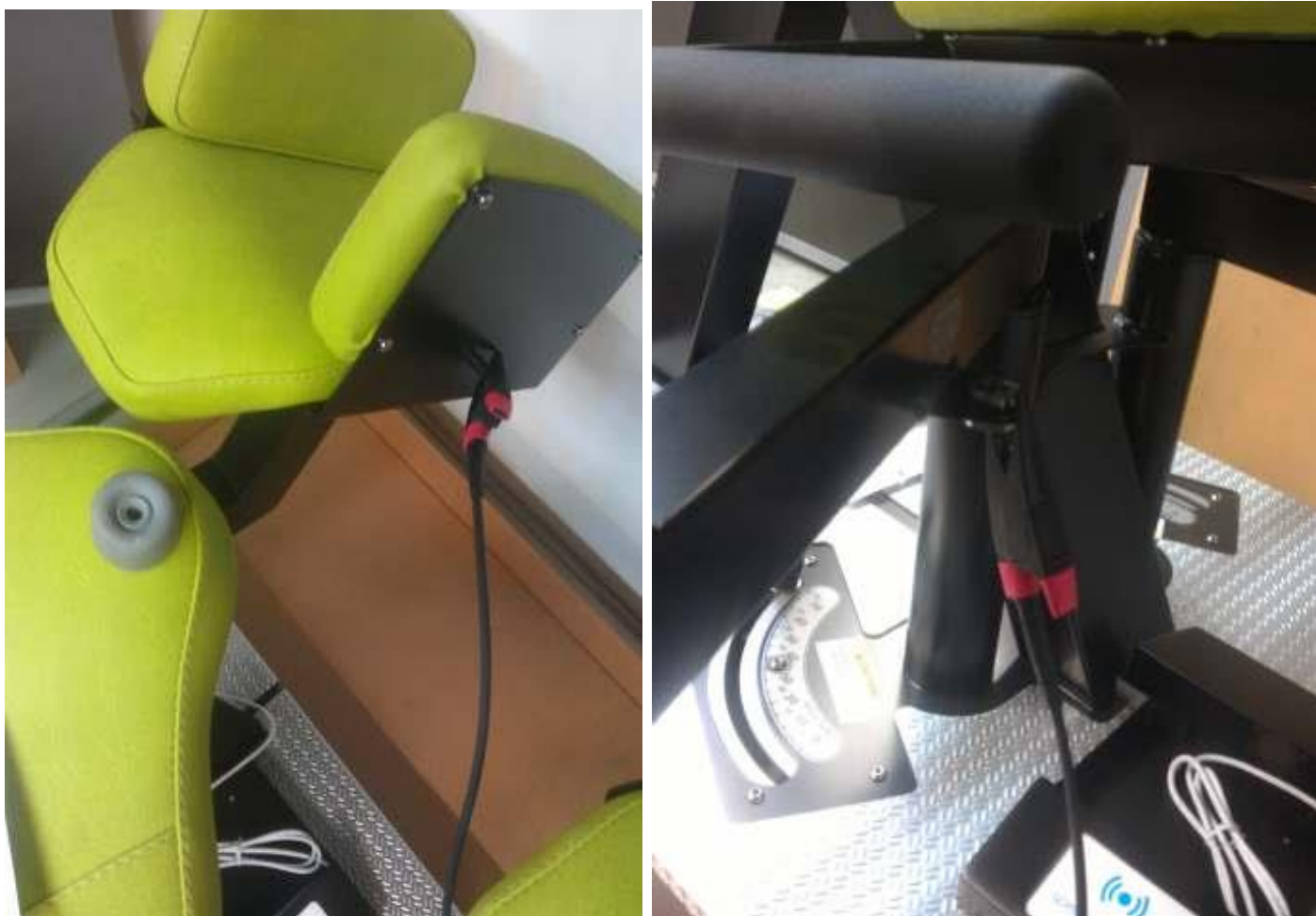
Figure 11, Attachment at the bumper pin and lever arm fixing point for force meter.
