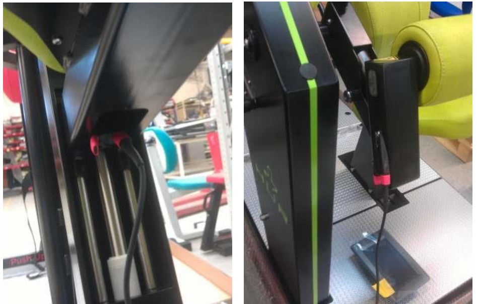
Figure 19, Attachment at seat motor bolt and lever arm fastening bolt.
