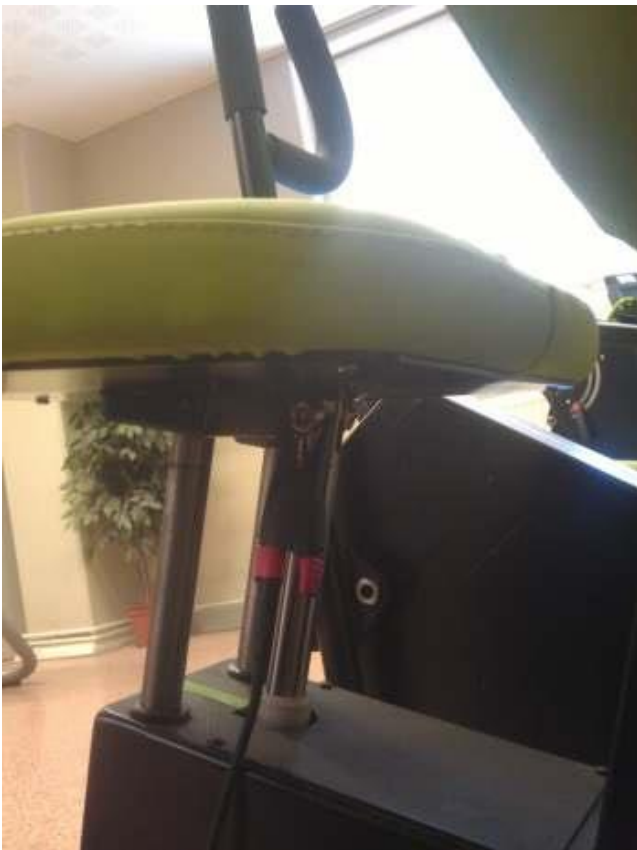
Figure 15, Attachment at seat motor bolt and levers fastening bolt.
