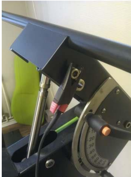
Figure 17, Attachment at seat motor bolt and levers cylinder bolt.
