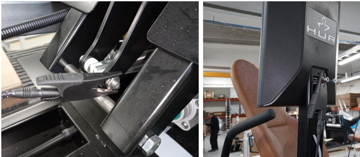
Figure 26, Attachment at back support adjuster motor bolt and display
