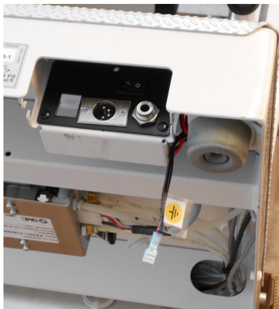
Figure 2, Ground reference connector with marking.
