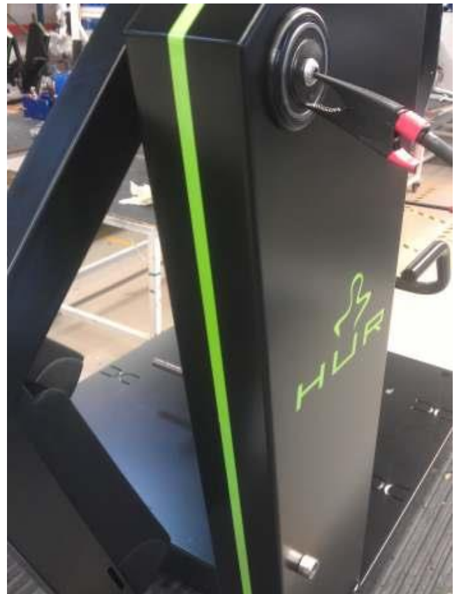
Figure 15, Attachment at seat motor bolt and levers fastening bolt.
